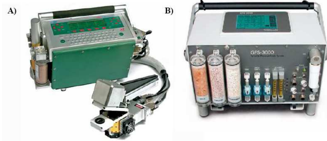
Figure 3.4. Li-6400 (A) and GFS-3000 (B) Portable Photosynthesis Systems
