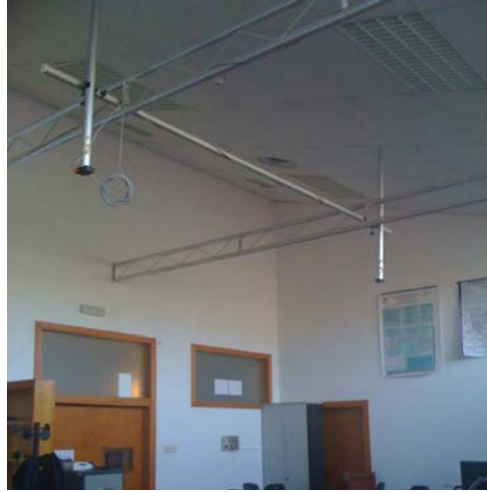
Figure 7.1: World-fixed cameras for ground truth calculation, on top of the picture
