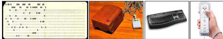
Figure 2.3: Examples of interfaces used for interacting with the computer: (a) punch card, (b) first mouse, (c) Microsoft keyboard, (d) Nintendo Wii remote.
