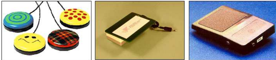
Figure 2.19: Switches for the hand, chin or foot.
