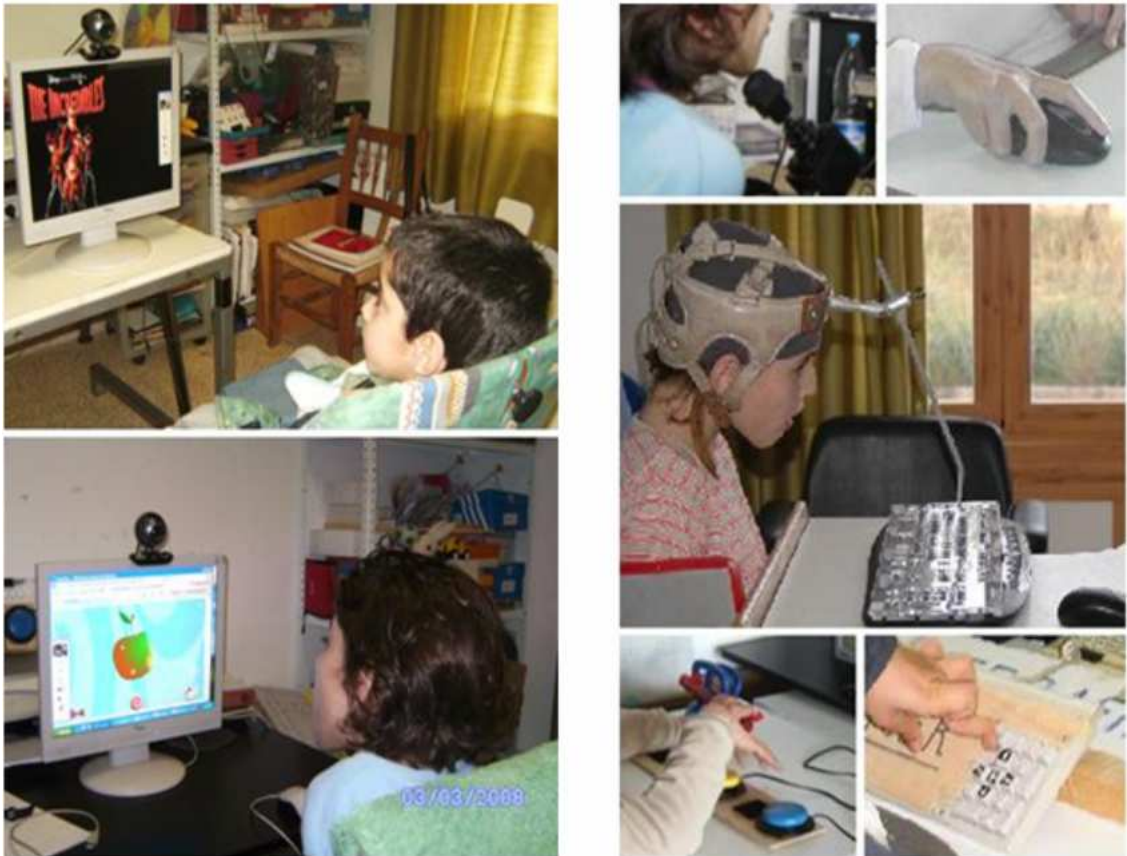
Figure 4.1: In the left column users are working with the hands-free interface. In the right column several other assistive tools which are also used: joystick held with the chin, mouse, head wand, switches and numerical keyboard.
