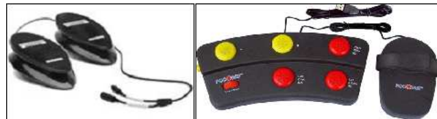
Figure 2.17: Feet systems: NoHandsMouse and Footime Foot Mouse.
