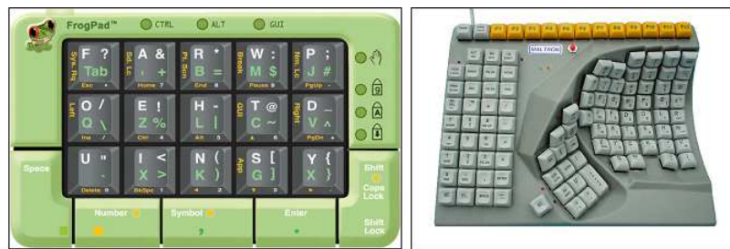
Figure 2.14: Frogpad and Maltron keyboards for one hand.
