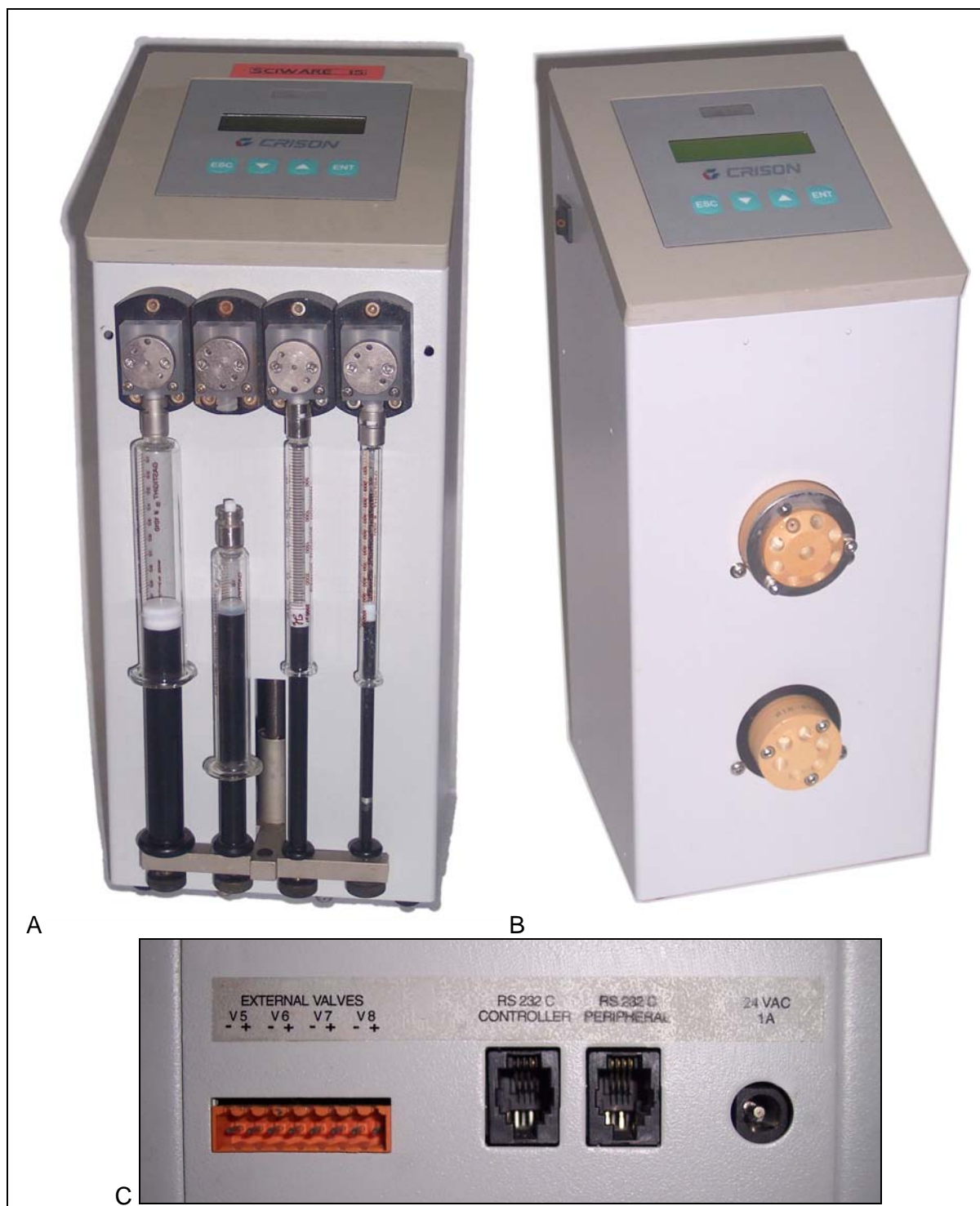
Figure 1: A: Multisyringe module equipped with glass syringes of 10, 5, 2.5, and 1 ml, the 5 ml syringe with loose Luer connection. B: Valve module with eight-port rotary selection valve (above) and low pressure six-port injection valve (below). C: Connections on the backside of the multisyringe device for RS232 control chain, power input and four additional external devices as solenoid valves (12V).
