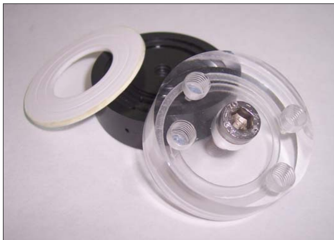
Figure 8: Trace-Trap debubbler cell with 1.5 mm thick PTFE membrane. The cell is equipped with two channels of different length.
