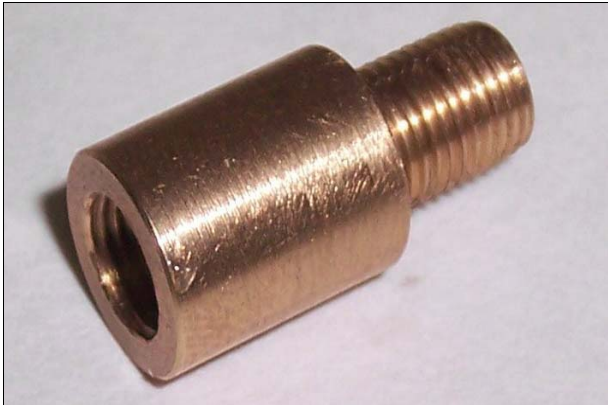
Figure 15: Spacer to be placed between optical fiber and light source to reduce the light intensity at the fiber tip by displacement of 2 cm. The spacer was made of bronze
