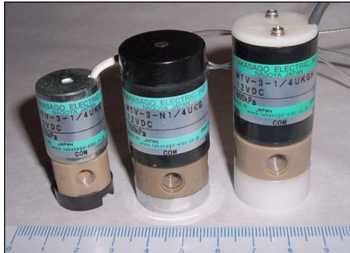
Figure 4: External multi-commutation solenoid valves (Takasago Electronic Inc.) used for flow manifolds. From left to right: STV-3-1/4UKG, MTV-3-N1/4UKG and MTV-3-1/4UKGH.
