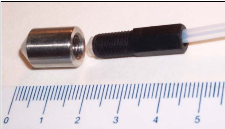
Figure 16: Tubing weight made of stainless steel used to assure the submersion of liquid reservoir tubing.
