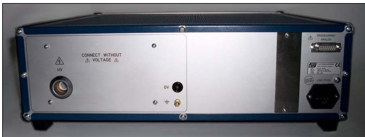
Figure 19: Back view of the high voltage power source HCP35-35000 with high voltage cable socket (left), ground socket (center), and analog control interface and power socket (right).
