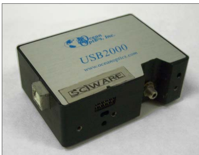
Figure 11: Miniature spectrometer USB 2000 used in this work. Connections for USB plug (left) and optical fiber (front) are visible.
