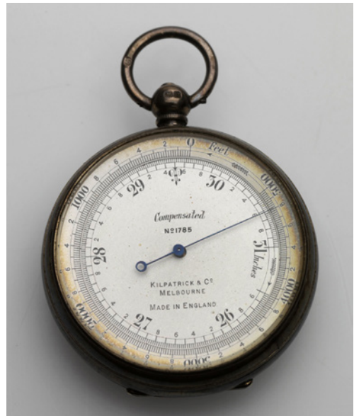
Figura 3: Altímetre de butxaca - Tipus baròmetre aneroide. Fitzpatrick & Co, Melbourne, circa 1900 (Museums Victoria Collections). https://collections.museumvictoria.com.au/items/1974454
