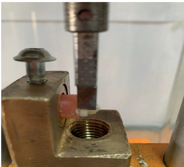
Figure 1: The shear bond strength test was conducted utilizing a universal tensile testing machine.
