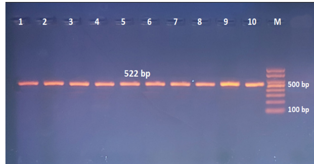
Figure 2: Enlargement of the human PIK3CA gene was obtained by 1% agarose gel electrophoresis and ethidium bromide staining. Conductive marker M: 100bp. the 522 bp PCR products in lanes 39 to 57.
