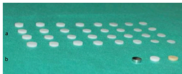
Figure 1: a. Translucent monolithic zirconia disks in different thicknesses, b. Titanium, white zirconia and yellow zirconia disks.
