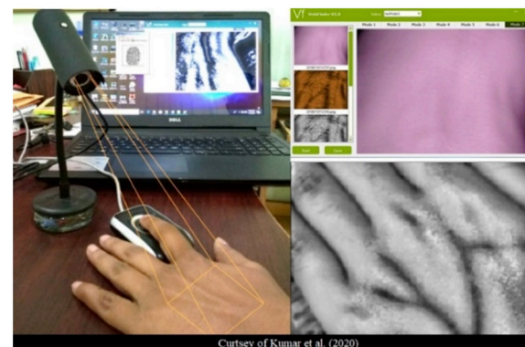
Figure 6: Dorsal hand vein acquisition using NIR camera VF620 26
