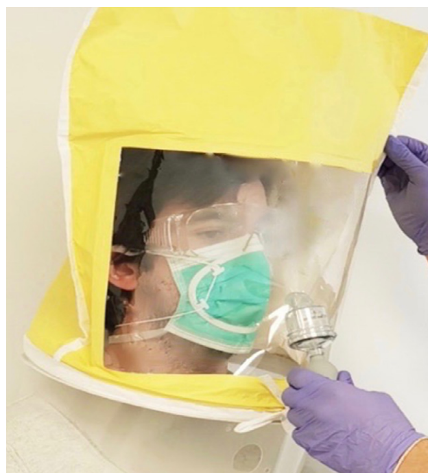
Figure 2: Subject with a type IIR surgical face mask with the AMS sealing device taking the qualitative fit test with the hood and nebulizer of the 3M FT-10 fit test Kit.
