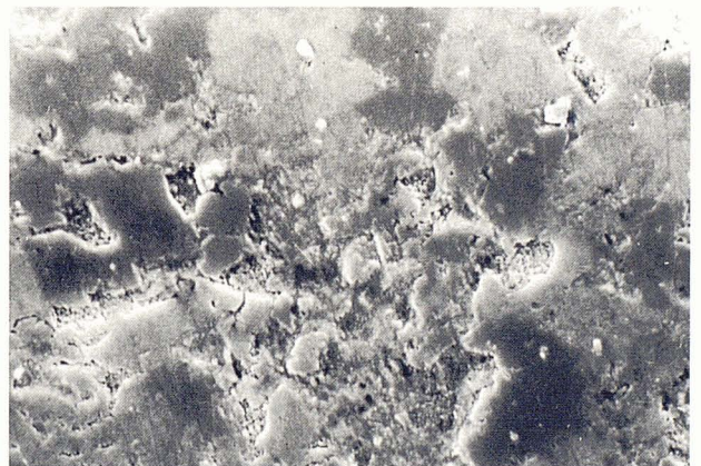
Figure 5: a) SEM showing surface area increase due to biological action (RK). Scale bars: 100µm and 20µm. b) Detail of polished surface of sample RP, showing irregularities which could be the incipience of a small quantity of carbonated particles. Scale bars: 100µm and 10µm.
