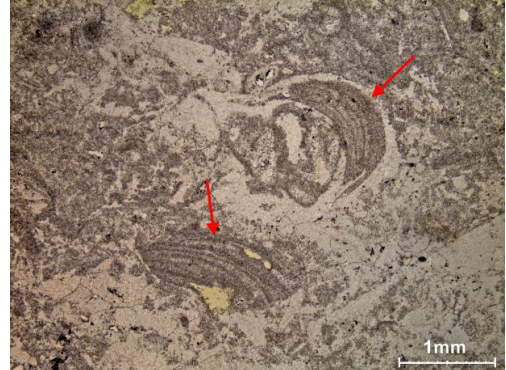
Fig. 5. Photomicrograph of the sample E22 (X1615). Largely recrystallized boundstone (coralline red algae still recognizable, red arrows) – Santa Monica I.
