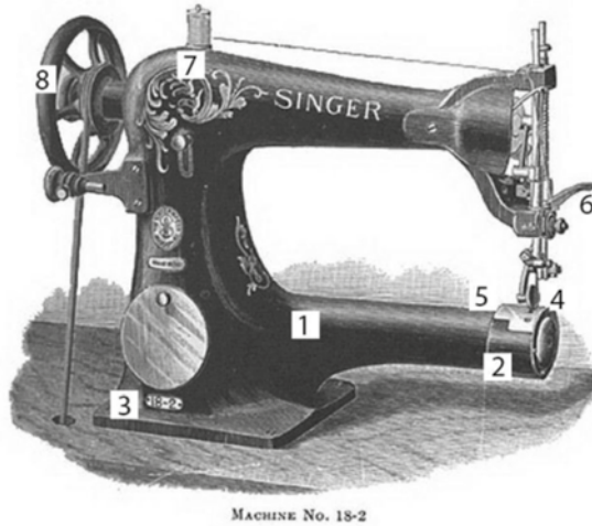
Fig. 4. Màquina de repuntar SINGER 18.2. Instructions for using and adjusting Singer sewing Machines of Class 28. The Singer Manufacturin.
